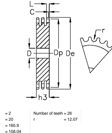
C = 2 D = 20 De = 165.9 Dp = 158.04 For chain size =  $3/4 \times 7/16$ For chain type = 12 B-3 h3 = 49.8 L = 10.8
